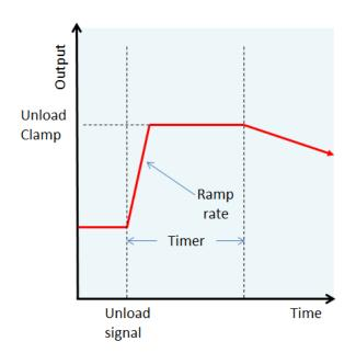
Ramp rates for all three MR stages were set to in affect step open the anti-surge valves with target opening positions 10 to 20 percent above their full recycle positions. Since the effect on the Propane circuit was less severe, the ramp rates for opening the anti-surge valves were more moderate and the opening positions were set close to their corresponding full recycle positions.
