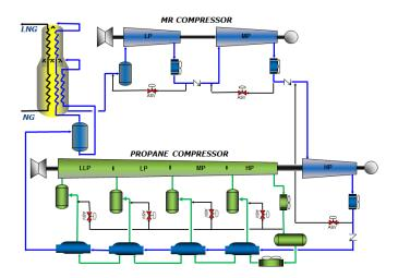
Conversely, when the MR circuit would trip, the HP stage had a sudden loss of flow and would surge due to the MR LP and MP anti-surge and bypass valves tripping open and the MP stage discharge check valve closing. In addition, the drop in MR flow through the propane chillers caused a loss of propane vapor production, requiring the propane compressor to counteract by quickly opening its anti-surge valves. The propane string would reach the gas turbine power limit and shutdown on underspeed.
