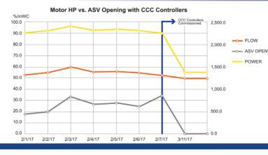
3. Motor power consumption by antisurge recycle control optimization
