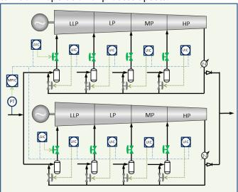
Fig. 4 - Constant Speed Parallel C3 Compressors
