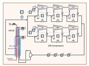
Fig. 5 - Parallel MR Compressors and MCHE
