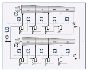
Fig. 2 - Parallel Load-Sharing Control System
