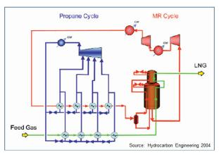
Fig. 1- Typical APCI C3/MR LNG Process
