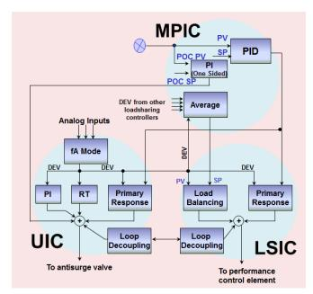
Fig. 3 - Load-Sharing Control Scheme
