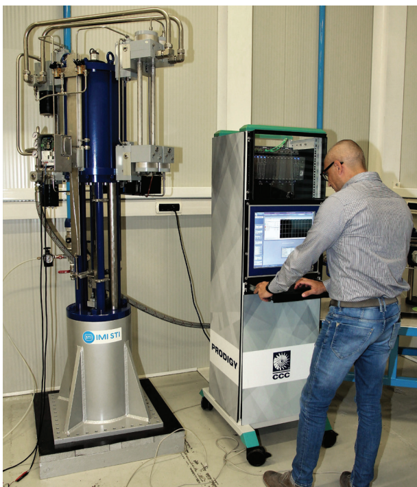
Figure 4. CCC Prodigy® control & IMI Critical actuation test bench.
