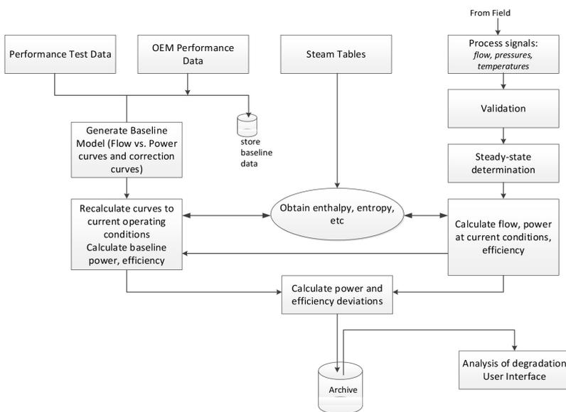
**Figure 3.** TPA simplified schematic.
