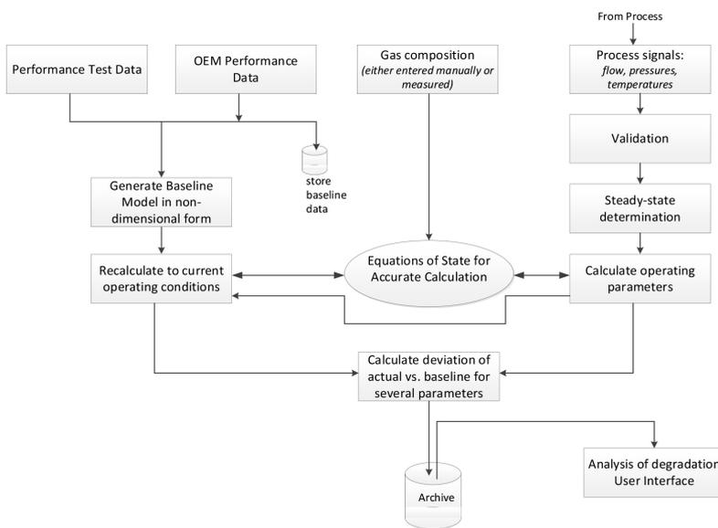
**Figure 2.** CPA simplified schematic.
