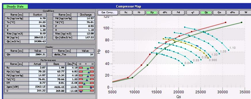
Figure 4. CPA typical operator and engineering interface screen.
