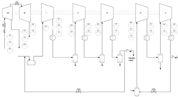
**Figure 1.** Five-stage charge gas compressor PFD at ENI Versalis Priolo.
