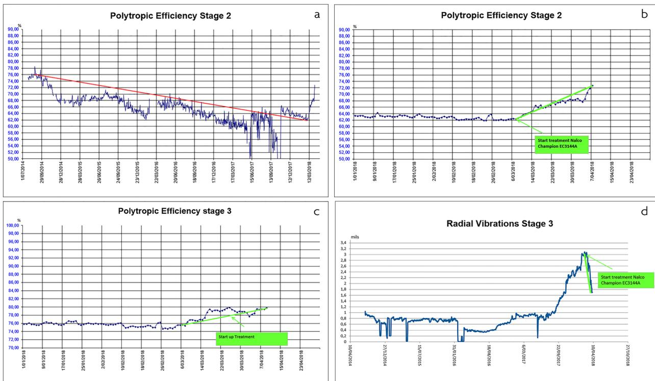
**Figure 6.** A and B illustrate stage two efficiency reduction before treatment/efficiency recovery after treatment, while C and D present stage three efficiency increase after treatment/vibration decrease after treatment. (A) Over 14% efficiency decline stage two. (B) Over 10% efficiency recovery stage two. (C) Over 4% efficiency recovery stage three. (D) Vibration decrease stage three.
